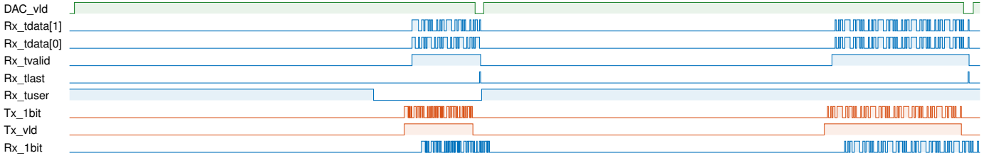
Fig. 8. Mixed-mode simulation results. The first packet is transmitted using QPSK, and the second packet is transmitted using BPSK.
